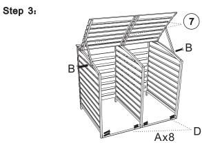
(1)Secure roof holder part⑦ on left and right panels, each with 1x screw(B).
