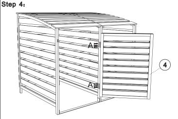
Secure each front door ④ and ⑤ with 6x screw(A) as shown, total 12x screw(A)here.
